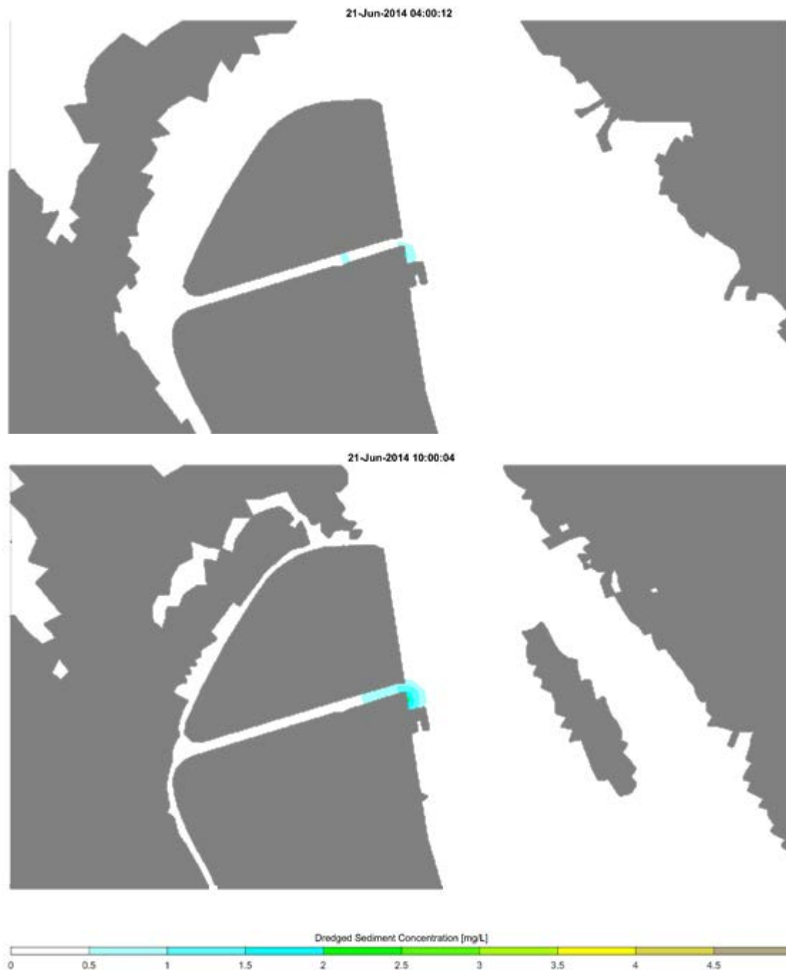
Figure 7.1 Typical tailwater plume depth-average TSS concentration (Top: neap flood tide, Bottom: neap ebb tide)
